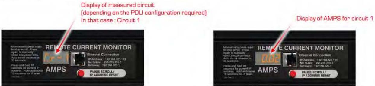
The display scrolls through the most recent current measurement (in AMPS) for each circuit, one at a time. It displays a circuit name, pauses and then displays the measurement. Momentarily press the red button to pause the display on the current measurement selected. The display will begin to scroll again 30 seconds after the last button push.
